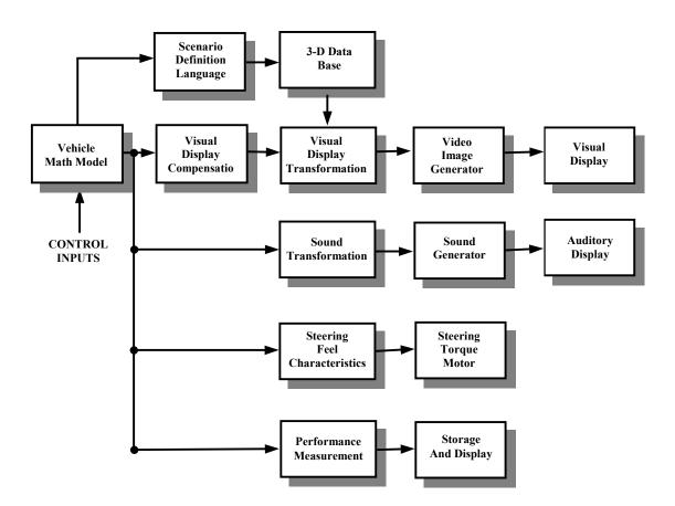
Figure 2: Functional Block Diagram of the Vehicle Dynamics Simulator
