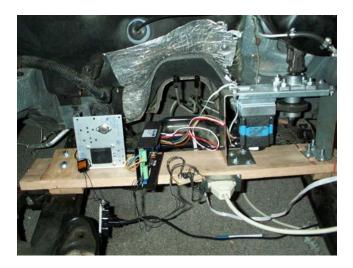
Figure 11: Full View of the Steering System
