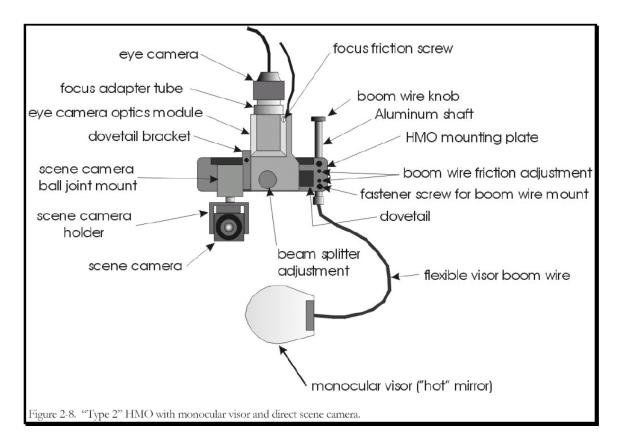
Figure 8: Head mounted optics (from the ASL Eye Tracking System Documentation)
