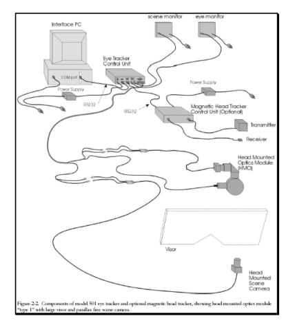
*Figure 7: Eye tracking hardware (from the ASL Eye Tracking System Documentation)*
