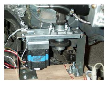
Figure 10: Partial View of the Steering System
