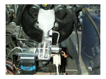
Figure 12: Components of the Braking System
