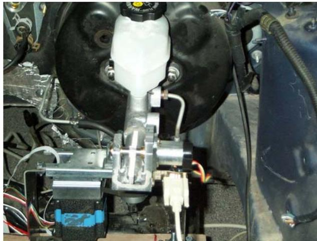
*Figure 12: Components of the Braking System*
