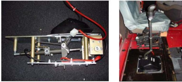
**Figure 6: Faros gear box system and final assembly in simulator cabin**
