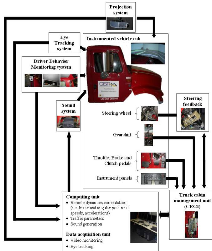
**Figure 1: CISR Truck Driving Simulator**
