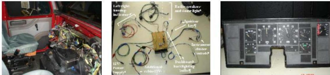
**Figure 8: Cabin instruments wiring, connecting interface, and instrument panel**
