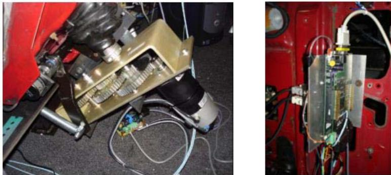
**Figure 5: Faros steering feedback system and INRETS control unit**
