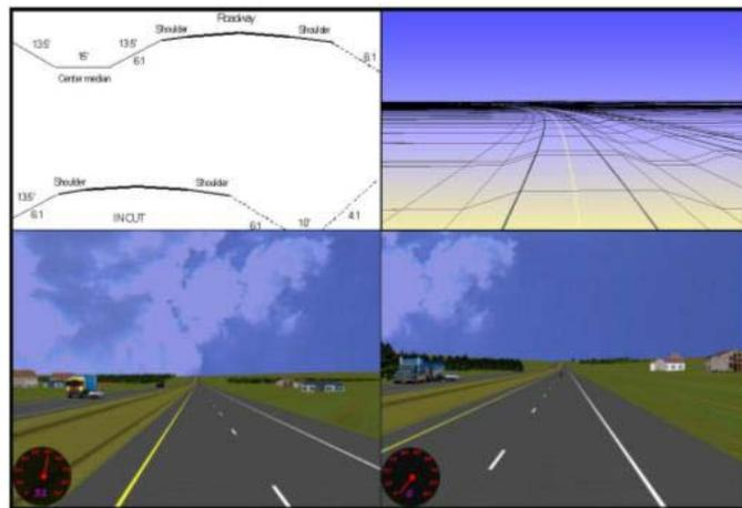
**Figure 9: Alignment data, 3-D mapping, and finalized driving scene**
