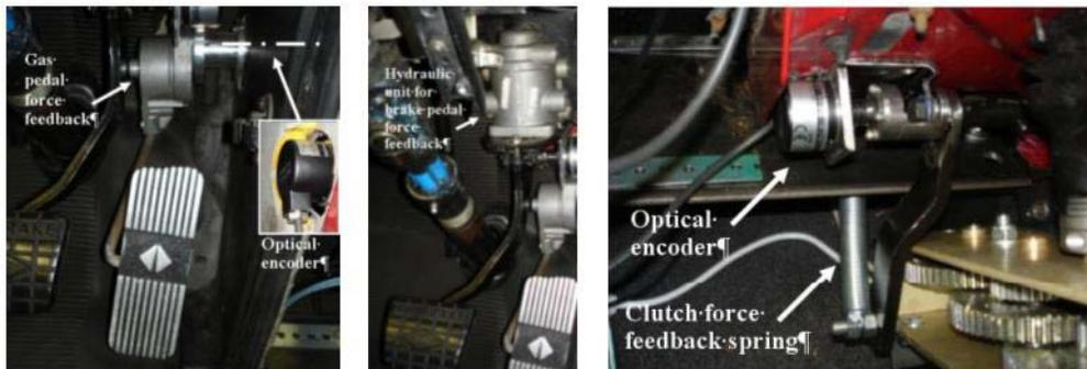
**Figure 7: Optical encoders mounted on the truck cabin pedals**
