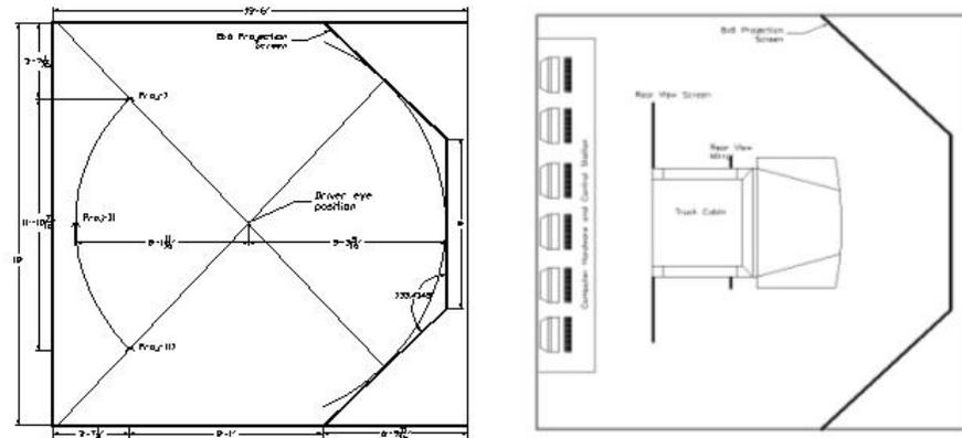
**Figure 2: General layout of the driving simulator display system**
