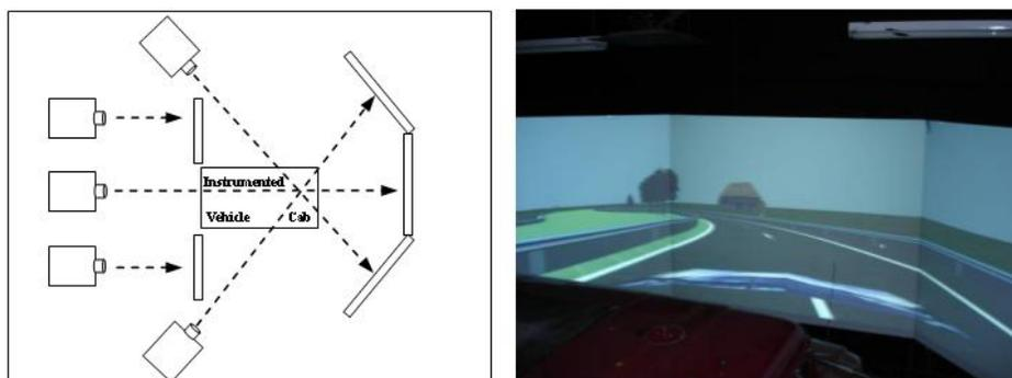
**Figure 4: Front and rear projection in the truck driving simulator**
